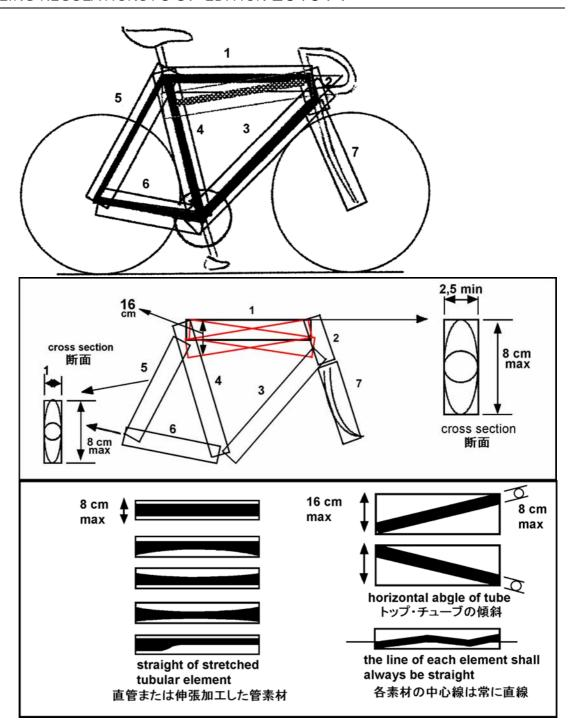
1.3.021 For individual time trials and for track competitions, the elements of the bicycle frame may be tubular or solid, assembled or cast in a single piece in any form (including arches, cradles, beams or any other). These elements, including the bottom bracket shell, shall fit within a template of "triangular form" defined in article 1.3.020. (See diagram "Shape (2)")
