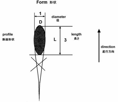
A fuselage form shall be defined as an extension or streamlining of a section. This shall be tolerated as long as the ratio between the length L and the diameter D does not exceed 3.
