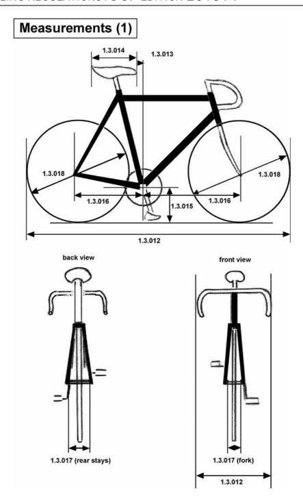
**1.3.012** A bicycle shall not measure more that 185 cm in length and 50 cm in width overall. 自転車は全長185cm以内, 全幅50cm以内でなければならない.
