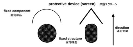
A protective screen shall be defined as a fixed component that serves as a windscreen or windbreak designed to protect another fixed element of the bicycle in order to reduce its wind resistance.
