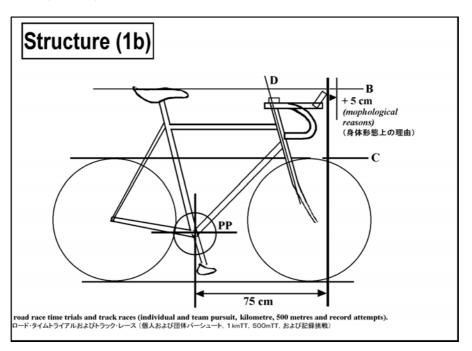
1.3.024 Any device, added or blended into the structure, that is destined to decrease, or which has the effect of decreasing, resistance to air penetration or artificially to accelerate propulsion, such as a protective screen, fuselage form of fairing or the like, shall be prohibited.
