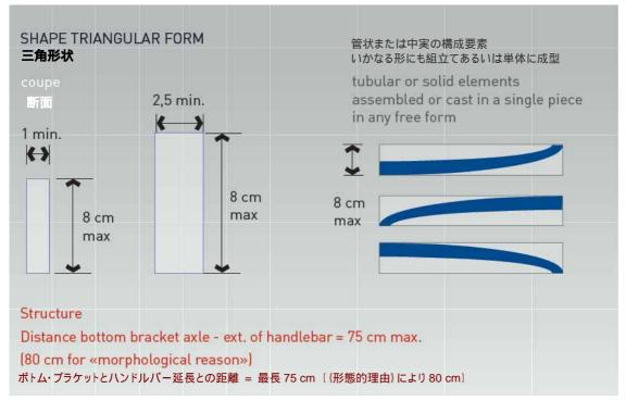
The profile of the extension must conform to the 1:3 ratio in accordance with Article 1.3.024. The extension must be fixed and not feature a system that would allow a change of length or angle during the race.
