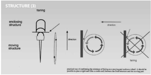
fairing shall be defined as the use or adaptation of a component of the bicycle in such a fashion that it encloses a moving part of the bicycle such as the wheels or the chainset. Therefore it should be possible to pass a rigid card (like a credit card) between the fixed structure and the moving part.
