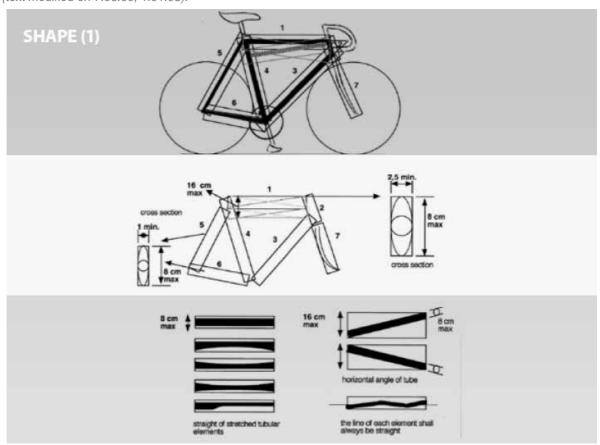
• 1.3.021 For road time trials and for track competitions, the elements of the bicycle frame may be tubular or solid, assembled or cast in a single piece in any form (including arches, cradles, beams or any other). These elements, including the bottom bracket shell, shall fit within a template of the □triangular form□defined in article 1.3.020. (See diagram «Shape (2)»).
