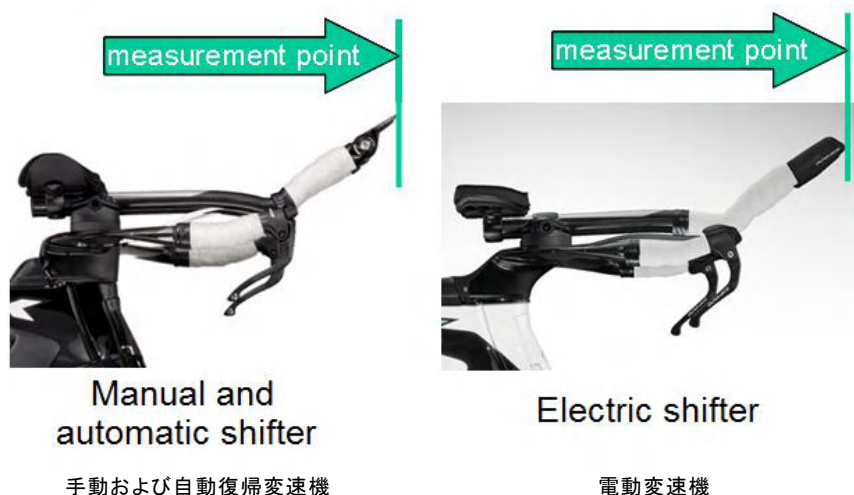
Figure 42: Point at measurement of 75 cm distance for different types of gear lever
