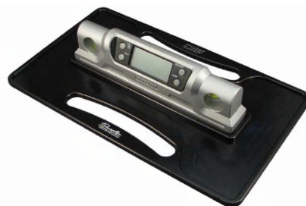
Figure 4: Official measuring device to check saddle inclination
