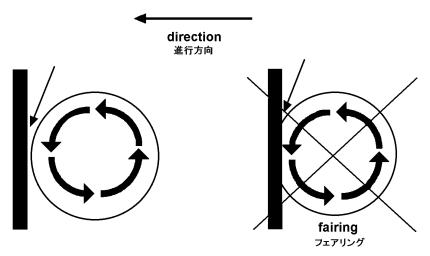
A fairing shall be defined as the use or adaptation of a component of the bicycle in such a fashion that it encloses a moving part of the bicycle such as the wheels or the chainset. Therefore, it should be possible to pass a rigid card (like a credit card) between the fixed structure and the moving part.
