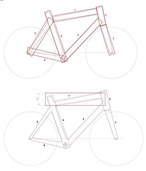
Tubes 1,2,3,4; 2.5cm minimum & 8cm maximum Tubes 1,2,3,4,: 2.5cm minimum & 8cm maximum Tubes 5,6,7: 1cm minimum & 8cm maximum
