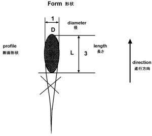
A fuselage form shall be defined as an extension or streamlining of a section. This shall be tolerated as long as the ratio between the length L and the diameter D does not exceed established dimensional requirements as defined in articles 1.3.020 (framesets), 1.3.022 and 1.3.023 (handlebars, base bars and fixed time trial extension).
