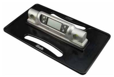
The reference value will always be the measurement of the angle of the incline of the saddle, but for events at which the official measuring device is not available, commissaires will measure the difference between the heights of the highest points of the front and rear of the saddle using a spirit level. The tolerance for the height difference is 1 cm. This value has been defined taking into account the mean distance between the highest points at the front and the back of the saddle.
