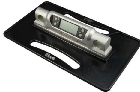
Figure 7: Official measuring device to check saddle inclination
