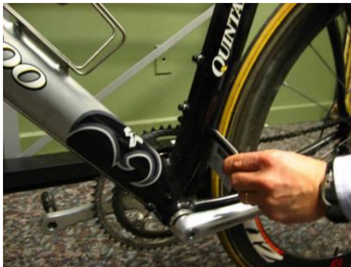
Figure 64: Insertion of a credit card between the wheel and frame to check that a fairing is not present
