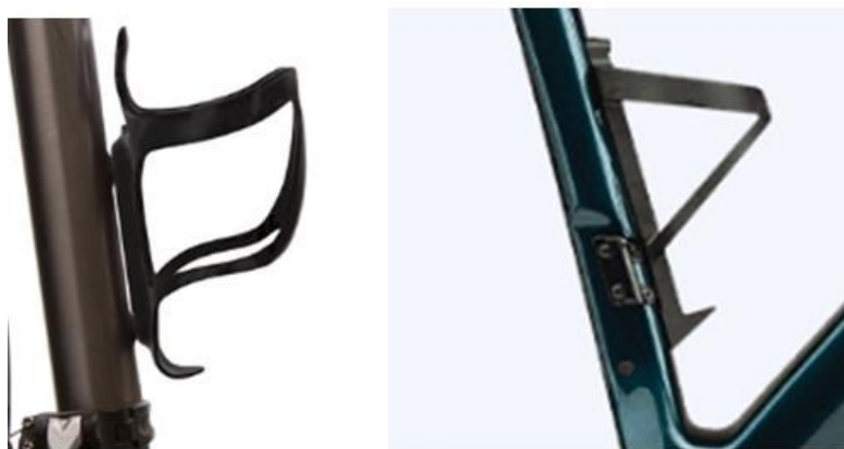
Figure 65: Illustration of a physical (left) and a visual (right) space between the bottle and the tube to which it is attached.
