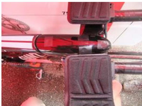
Figure 4: Illustration of the addition of the adhesive tape to cover bolts access
