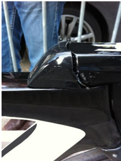
Figure 58: Cover added to frame to conceal brake cables
