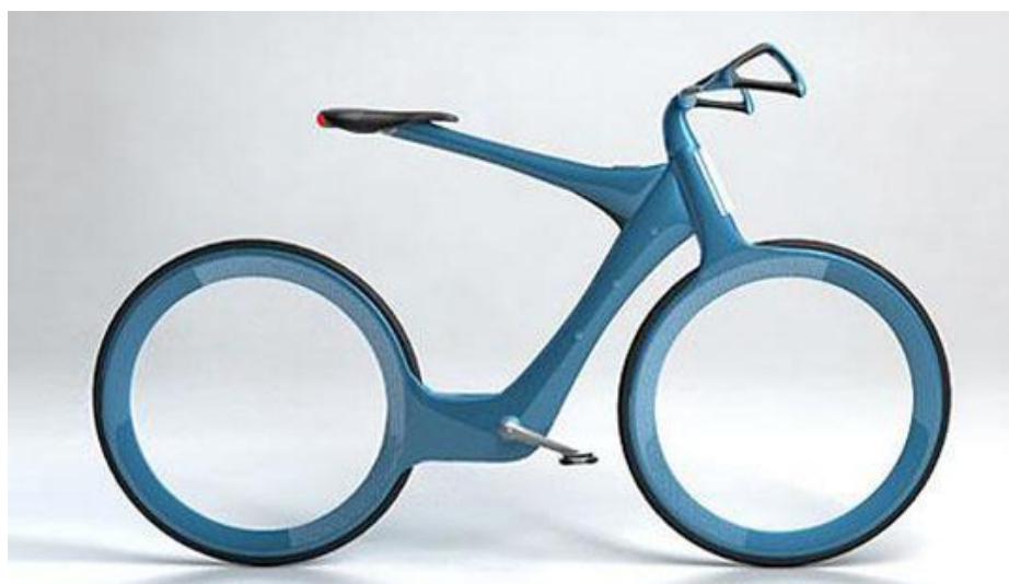
Figure 11: Example geometry of a bicycle that does not comply with UCI regulations 図 11: UCI 規則に従わない自転車の形状例
