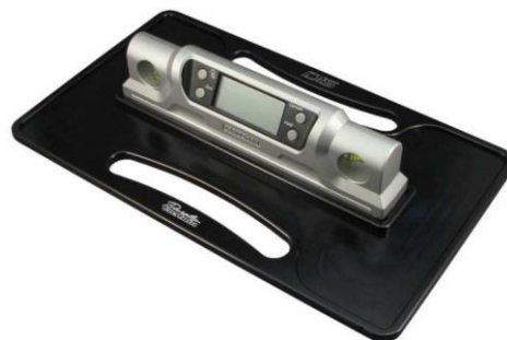
Figure 6: Official measuring device to check saddle inclination
