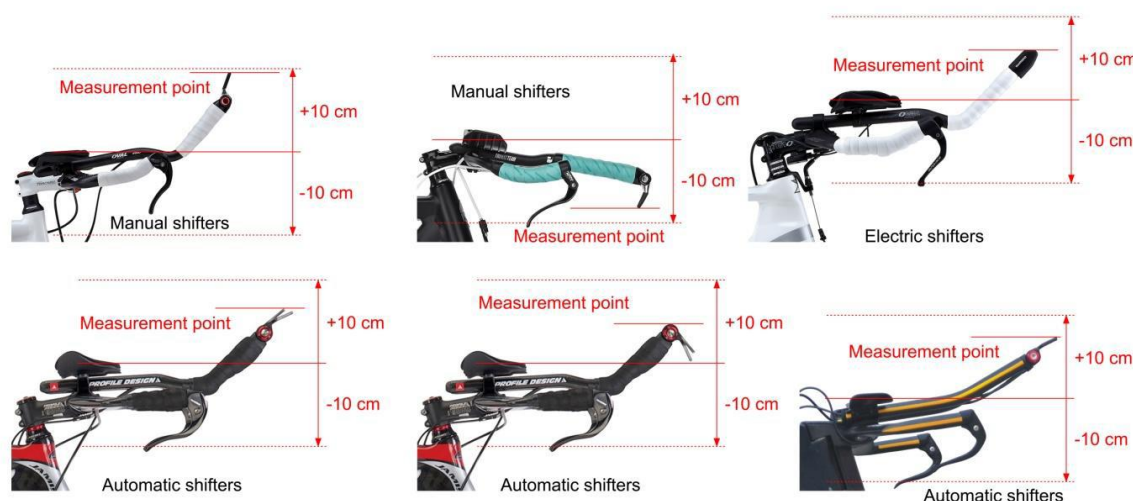
Figure 46: Points of measurement for the vertical limits of the handlebars extensions and any accessories
